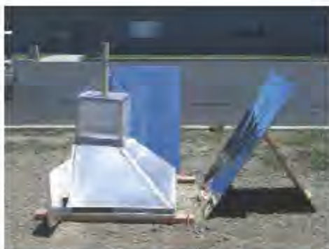
Because many areas have limited daylength and light intensity, researchers are working with collaborators in Tanzania to use mirrors to create a concentrated solar dryer for tomato and mango.
